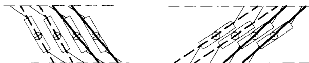
Figure 4. A schematic of conformational-driven inversion phenomena in ferroelectric systems. The bold dashed lines indicate the optical axis of the molecules, while the full lines show the mass axis.
